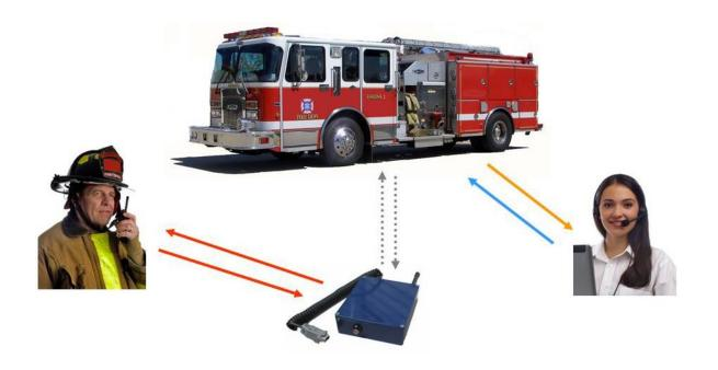
Portables don't talk as far as mobiles? If that's a problem, just connect the BlueBox-PTX to your existing VHF, UHF or 700/800 MHz mobile radio. Then your portable, even low cost models, can communicate as far as your mobile! The cost? Just \$949 and it's plug and play compatible with most mobile radios. No wiring or drilling required! For more information, check out <a href="http://info4u.us/BlueBox-PTX.pdf">http://info4u.us/BlueBox-PTX.pdf</a>
