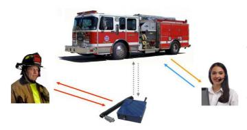
Operationally, the *MobileLink* system works in the same way as the *DoubleTalker* system. The main difference is that any VHF or UHF analog portable radio can be connected to most any mobile radio, whether analog or digital, in any frequency band from 20 to 800 MHz.
