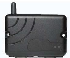
We call this the *Harkener*. Similar in size to the *Hornet*, the main difference is in the way it activates a call for assistance. The *Hornet* relies on a person pushing a button. The *Harkener* is activated by an electronic switch closure of an associated device such as a home or business security alarm system, activated by a motion sensor, smoke detector or associated wireless call buttons.
