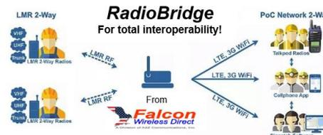
**RadioBridge** provides the ability for different types of radios to talk to each other, like allowing low cost analog VHF radios to talk to pricey digital P25 radios. A good example of how this technology works is [info4u.us/DavidKnows](http://info4u.us/DavidKnows) or linking P25 trunked radios to inexpensive UHF school radios. See [info4u.us/HaroldKnows](http://info4u.us/HaroldKnows).
